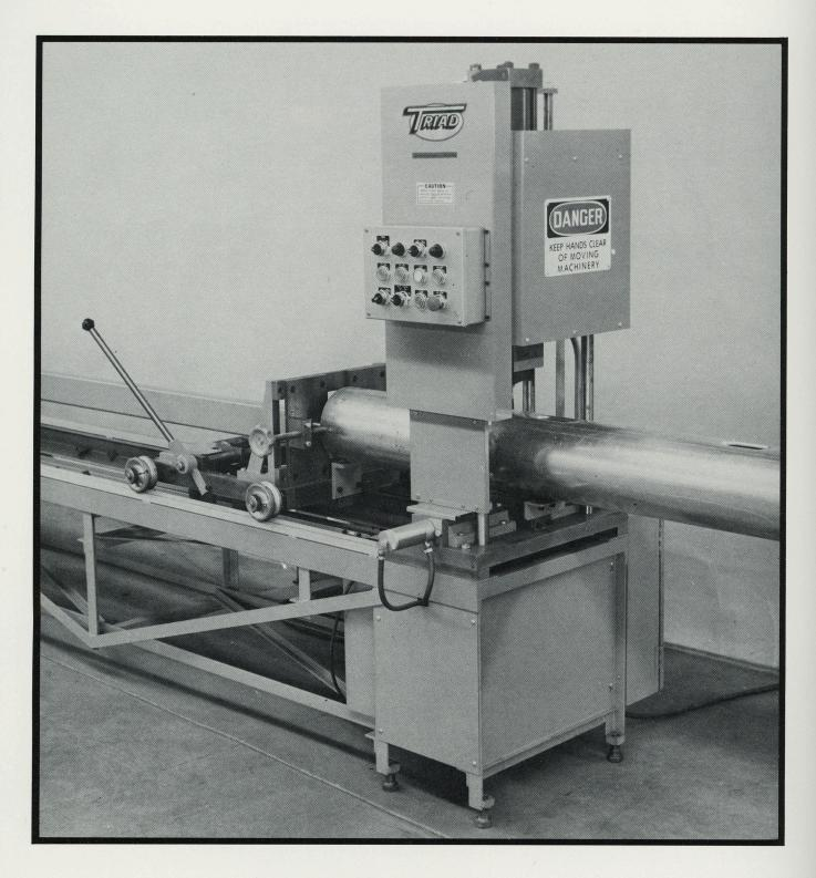
The TRIAD Gate Hole Puncher is a rugged machine designed for fast, efficient, safe, economical punching of holes in pipe up to 40 Ft. long. Also TRIAD's Puncher automatically spaces holes at desired settings in 6, 8, 10 and 12 inch diameter pipe with or without couplings. Eliminating mis-aligned dies or dangerous router bits with no more burrs to file, reduces set-up time and accomplishes this with semi-skilled labor!
