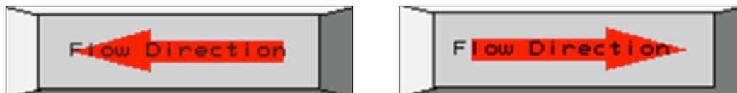
At the top of the screen there are 2 arrows to indicate what direction the water is currently flowing. If the water is flowing right, the top right "Flow Direction" arrow will be green. If the water is flowing left, the top left "Flow Direction" arrow will be green.
